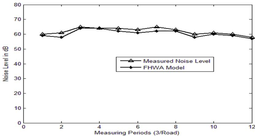
**Figure 4:** The FHWA in Comparison with the measured noise level
