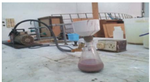
Plate 3: Gum Arabic Refining Set-up
